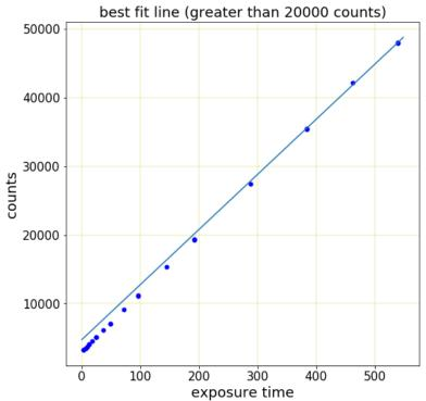
The counts/pixel increases approximately linearly with exposure time, although it does begin to flatten a bit as the counts/pixel increases past 20,000.
