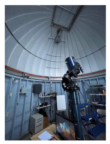
In order to use the telescope, we need to perform two operations to the dome. First, we need to open the dome shutter at the start of the night. Second, in order to see objects in different parts of the sky, we need to rotate the dome so that the opening points in the same direction as the telescope.
