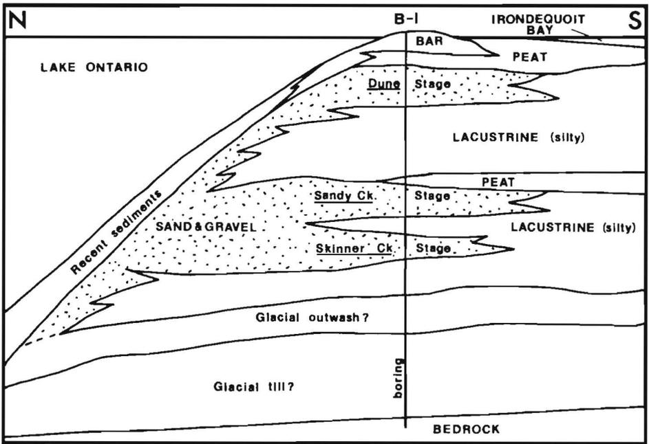
FIGURE 5: Diagrammatic north-south section through Irondequoit Bay bar to illustrate hypothetical facies relations created by rising lake stages as barrier bar grew by longshore transport. Development and stabilization of bar created lagoonal environments in bay, accounting for organic horizons. Vertical scale similar to Figure 4; horizontal scale diagrammatic only.
