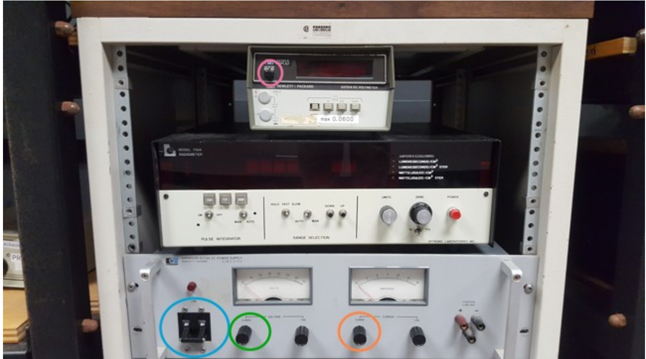
Figure 3: The power supply used to control the output of the lamp
