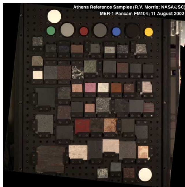
Figure 22. Pancam color composite image of rock target imaged during standalone camera thermal vacuum testing at -55^{\circ}\text{C} . This is a rotated subframe of a full 1024 \times 1024 image and was obtained using the MER-1 left Pancam (S/N 115). Pancam bands L4 (602 nm), L5 (535 nm), and L6 (483 nm) were used to generate an RGB composite simulating true color. The target was \sim 2.3 m from the camera.
