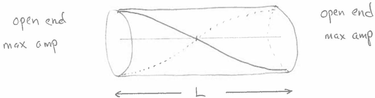
So, for example, a tube of length  $L$  open at both ends is shown above. A standing wave in the tube must have maximum amplitude at both ends; in other words, must have an anti-node at each end.
