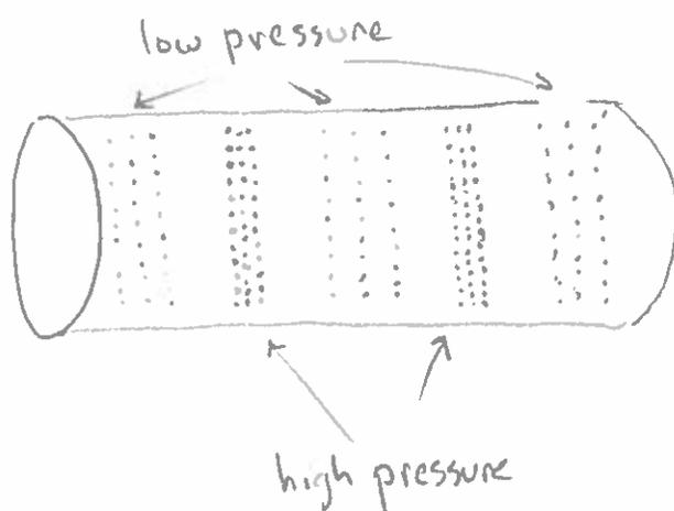
A sound wave inside the tube means that the pressure of air varies from place to place, and as a function of time.
