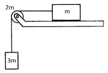
a) Find the acceleration of the system when released from rest, as a multiple of the gravitational acceleration *g*.
