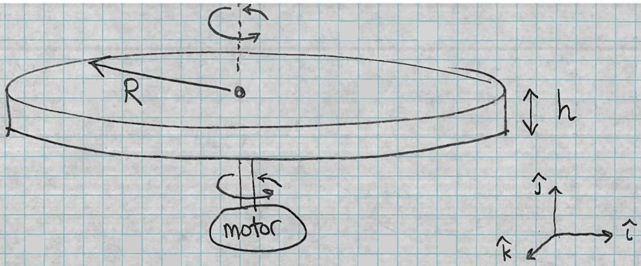
Potter's wheel has  $R = 0.4\text{ m}$ ,  $h = 0.05\text{ m}$ ,  $\rho = 7780 \frac{\text{kg}}{\text{m}^3}$ .
