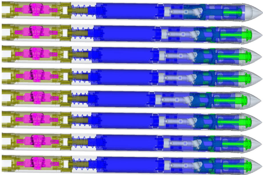
Fig. 5 Phases of a hammering cycle (top to bottom, cf. Lichtenheldt et al. (2014)) showing the interaction between the hammer (green), the suppressor (blue), and the outer hull (grey). (1) Mechanism fully tensioned. (2) The hammer is released and impacts the tip, providing the first stroke. (3) Recoil movement of the suppressor, compressing the brake spring. (4) Recoil movement of hammer and suppressor away from the tip. (5) Suppressor point of reversal is reached. (6) and (7) The brake spring and gravity drive hammer and suppressor tipwards, providing a second stroke. (8) Mechanism at rest
